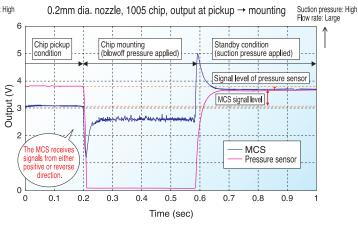
Compact and lightweight allows the flow sensor to be installed anywhere and also just above the nozzle (direct mounting onto the air tube between nozzle and ejector), enabling the high response for detection of pickup.
