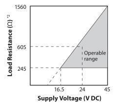
Figure 3. Supply voltage for travel transmission vs. load resistance characteristic
