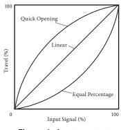
Figure 4. Input-output characterization
