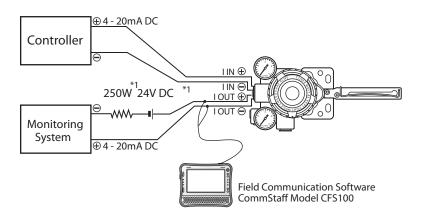
Figure 2. Positioner with travel transmission function (model AVP301)
