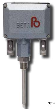
The BETA Temperature Switch is a pressure switch enclosure incorporating a sealed 2-phase (vapor/liquid) temperature sensor. When the temperature of the process increases, the vapor pressure of the liquid also increases.
